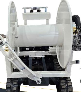
The TJR is provided with two threaded hose towing points where 1" & 1 1/4" hose from a jetting vehicle can be connected allowing the hose to be towed behind the TJR to its operating location.
